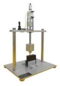
Mandrel: minimum 38mm long by 6.4 mm diameter Junction box fixture: adjustable Load force: 44.5N
