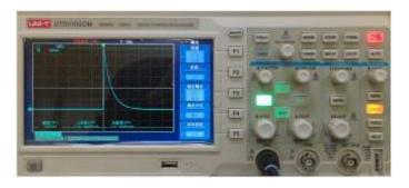
T = Time width of rated voltage from 30% to 90% Front time T1 =  $1.67 \times T = 1.2 \mu s$ Pulse width T2 = 50 $\mu s$  (time to half rated voltage value)
