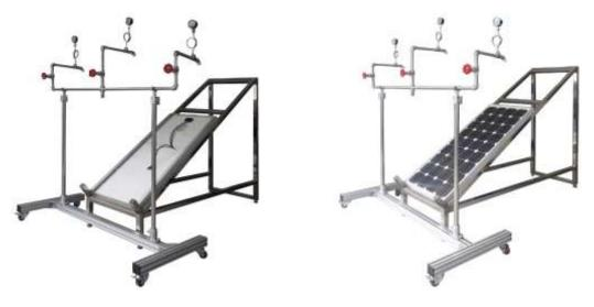
Module mounting angle 35 ° with the horizontal plane. The exposure time is to be 1h to the back and front of module. Test pass criterion: wet leakage current test
