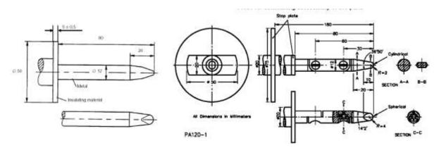
Application in VDE 0126-5 and VDE 0126-3, junction box and connector test conditions are as follows: 1. Fixing of lid at rewireable junction box - Screwless fixing of lid: Enclosures shall be tested with the test probe 11 according to IEC 61032 applied with a force of 75N for one minute to all points where this could cause a loosening of the lid. During test the lid shall not come off.
