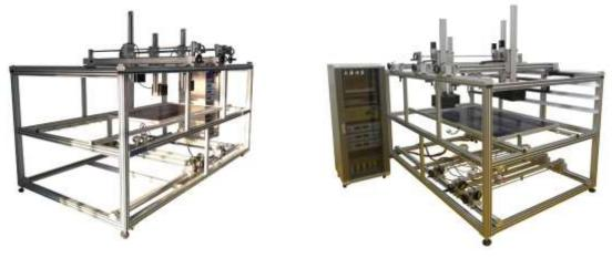
Light: LED lamps, small Calorific value, to avoid the battery temperature exceeds NOCT Center shaft two sets LED lamps, solved a technical problems of measuring cells in the same column. Light source horizontal and vertical displacement: transmission system
