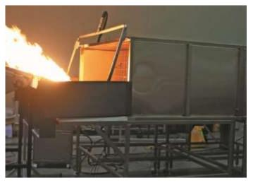
the test flame, such that the flame impinges only on the top surface of the module or panel.
