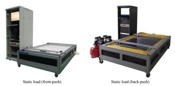
The new design, convenient operation, Pressure more evenly, 0~+100Pa @ 2400Pa Load mode: unidirectional or bidirectional Pressure regulation: an external air compressor is connected with a pressure regulating valve Electrical continuity measurement system: contain PC, DC 80V/5A power, PLC, Software.
