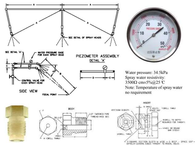
Test spray heads material: Molded nylon rain (see UL 1703)
